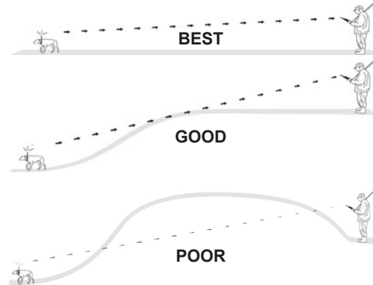
Line-of-Sight Radio Communication
